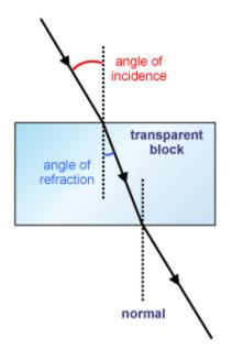
The speed of light waves depends on the material they are travelling through
