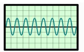
A high pitch sound on an oscilloscope (many waves per second) \* short wavelength
