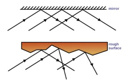
The angle of incidence = the angle of reflection
